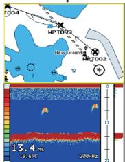
SmarterTrack combo sounder version offers a full featured 50/200KHz internal sounder compatible with a range of 600W Airmar transducers.
